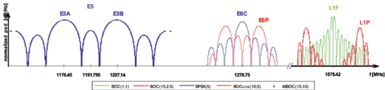
FIGURE 1B. Normalized Galileo Power Spectral Densities
