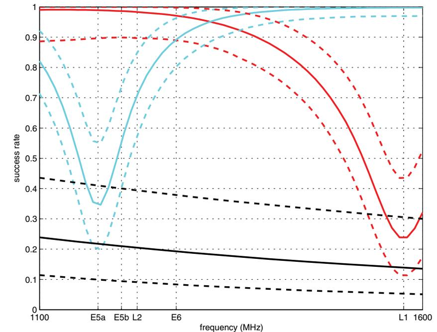
**FIGURE 1.** Mean, minimum, and maximum success rates during the day with Galileo. Black represents single-frequency; red, dual-frequency with one frequency fixed to L1; Blue: dual-frequency with one frequency fixed to E5a.
