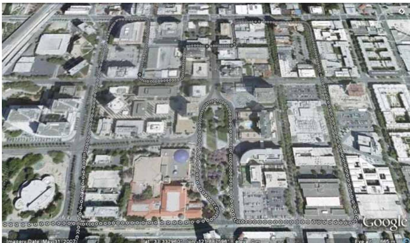
FIGURE 12 GPS+SBAS+GLONASS performance in San Jose, California
