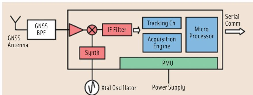
FIGURE 1 Schematic of a GNSS receiver inside a consumer product
