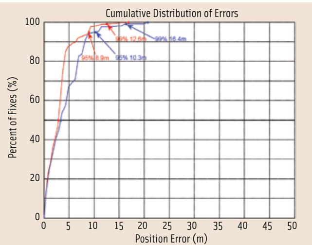
FIGURE 14 Comparison of GPS+SBAS (blue line) and GPS+SBAS+GLONASS (red line) CDF of errors in San Jose Urban environment
