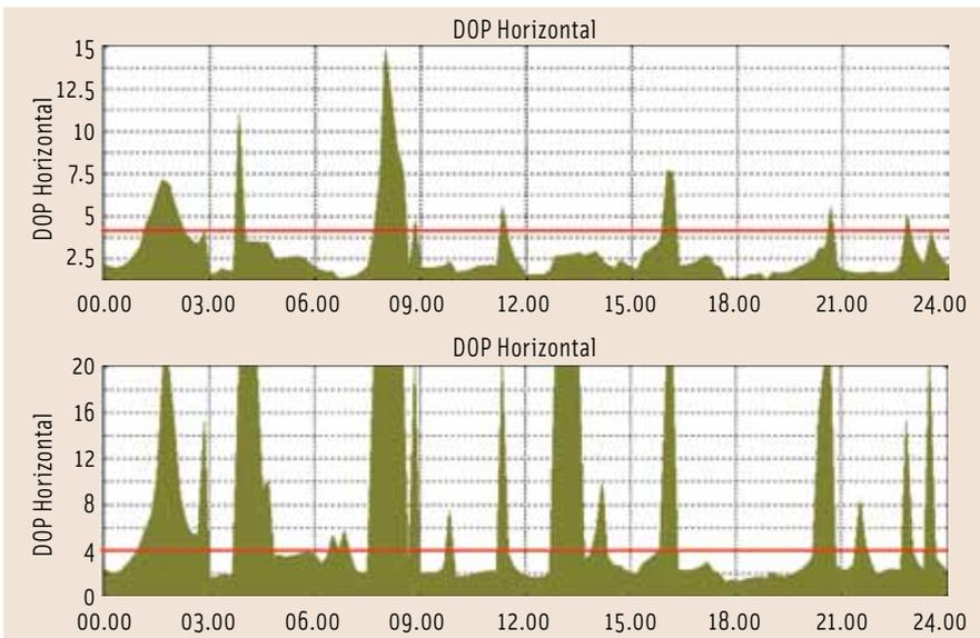
FIGURE 5 HDOP values in simulated Tokyo test with a GPS-only receiver (bottom graph) and GPS plus SBAS and QZSS (top graph)
