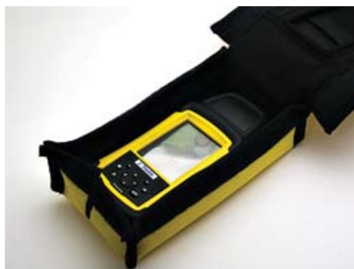
Custom insulated bag (left) with main access flap open. (at right) Insulated bag with main flap closed and heating element installed in the open screen cover. Photos by Edward Wingate
