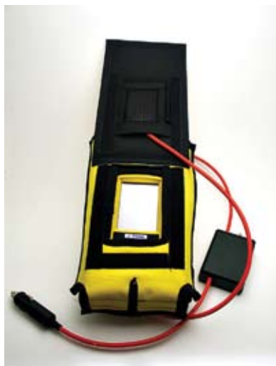
Custom insulated bag (left) with main access flap open. (at right) Insulated bag with main flap closed and heating element installed in the open screen cover. Photos by Edward Wingate
