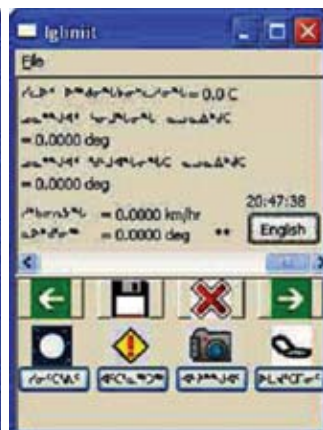
FIGURE 3 Igliniit interface showing the sixth page as displayed in Inuktitut. Pressing the English toggle button switches the interface back into English language mode
