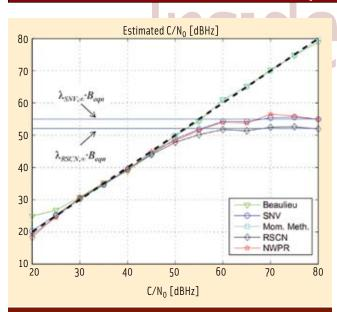
FIGURE 2 *C/N*<sub>0</sub> estimates for  $\sigma_{\theta}$  = 1° The dark dashed line indicates the true *C/N*<sub>0</sub> values.
