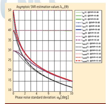
FIGURE 3 Asymptotic SNR estimates vs. the phase noise standard deviation.
