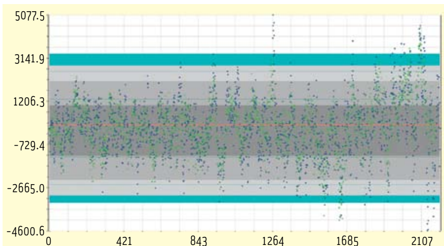
FIGURE 3 Vertical scatter diagram using the original pseudo-ranged data (1 s, blue dots) and the interpolated 30-s dataset (yellow-green dots). Empirical 68%, 95% and 99% confidence intervals are indicated in shades of gray for the interpolated data and in cyan for the original data set (y-axis in units of millimeters, x-axis in seconds).
