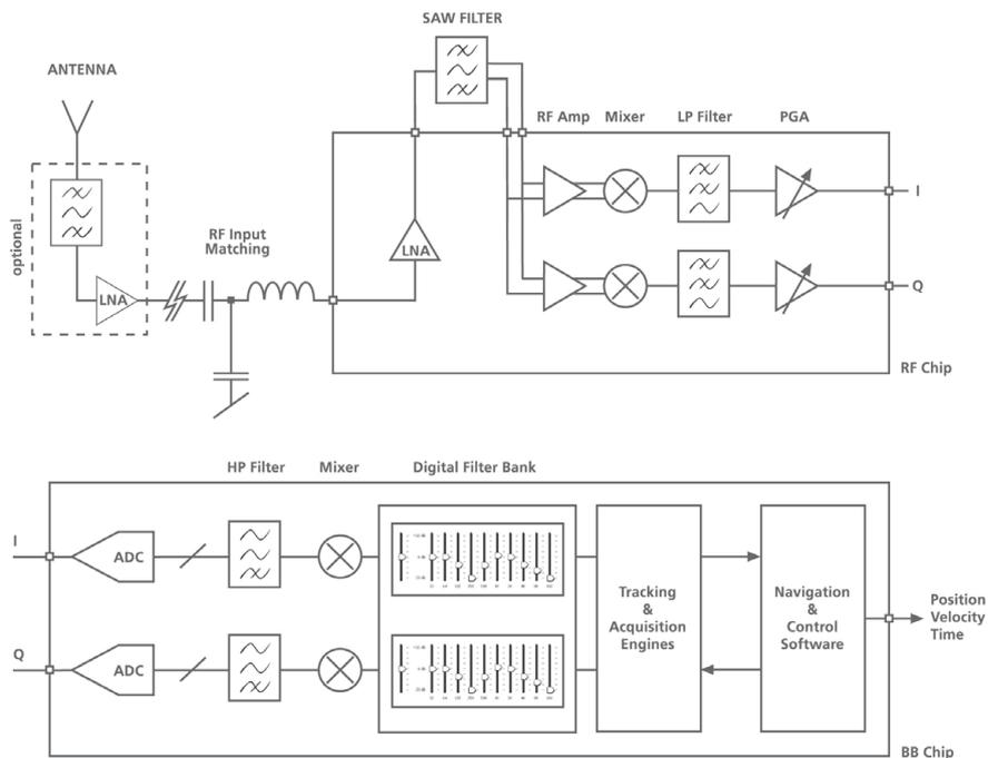
Figure 1: This simplified block diagram of a GPS receiver based on the u-blox 5 / 6 technology shows the SAW filter at the signal input to block out-of-band interference plus the software-controlled digital filter bank that blanks out specific interference sources.
