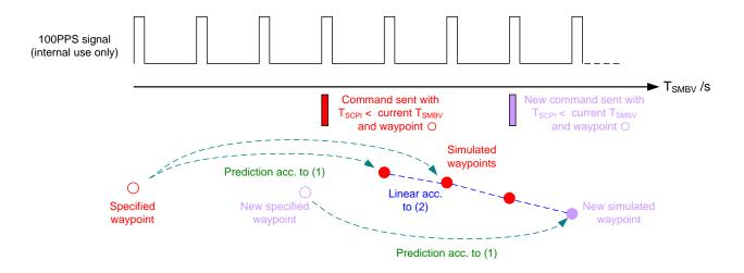
Every 10 ms, the SMBV extrapolates the position coordinates according to the same third order polynomial (i.e. formula (1)) until it receives a new HIL command with new position coordinates.
