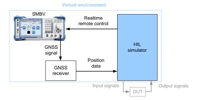
Most GNSS simulators support moving receiver simulation but only with predefined trajectories, i.e. the movement of the receiver is entirely predetermined. For HIL applications however the movement of the receiver must be controllable in real-time. This means the GNSS simulator must support realtime update of the simulated trajectory.
