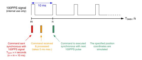
Assuming a HIL command is sent out synchronous to the SMBV's internal 100PPS signal at a time point that corresponds to  $T_{SMBV} = m$  seconds. This command includes a  $T_{SCPI}$  of n seconds where n is m + 10 ms. The HIL command is received and evaluated by the SMBV. This takes maximally 5 ms. The execution of a HIL command is always synchronous with the internal 100PPS signal. This means, the specified position coordinates are simulated at the next upcoming 100PPS pulse.
