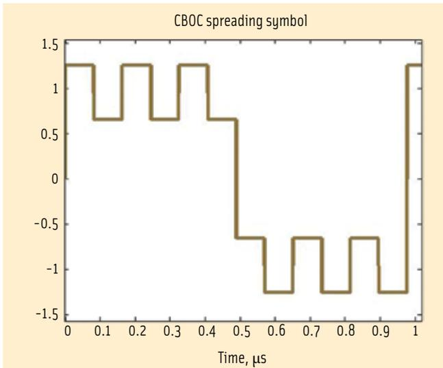
FIGURE 1 The spreading symbol of CBOC is made by algebraic addition of BOC(1,1) and BOC(6,1) spreading symbols.
