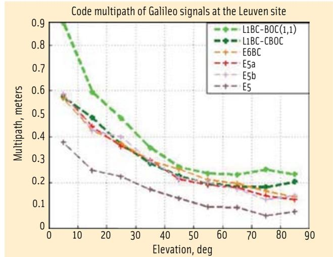
FIGURE 3 Standard deviation of code multipath for Galileo signals transmitted by GIOVE-B. The two thicker lines indicate L1BC modulations: BOC(1,1) in light green and CBOC in dark green.
