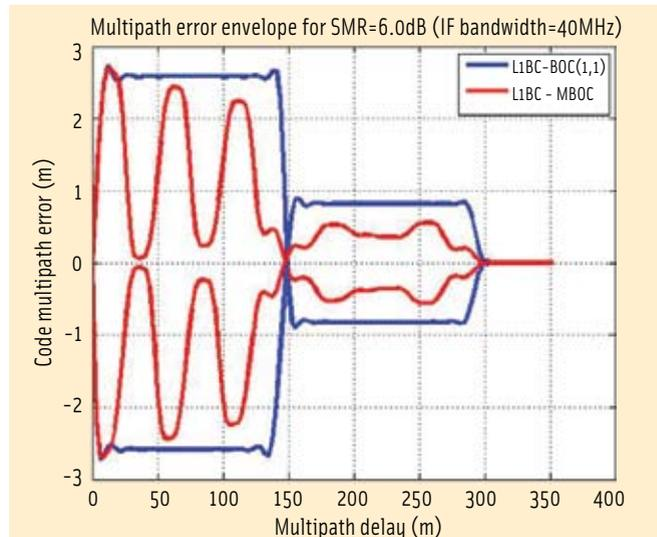
FIGURE 2 Multipath error envelopes of MBOC versus BOC(1,1) computed at a signal/multipath ratio of 6 dB
