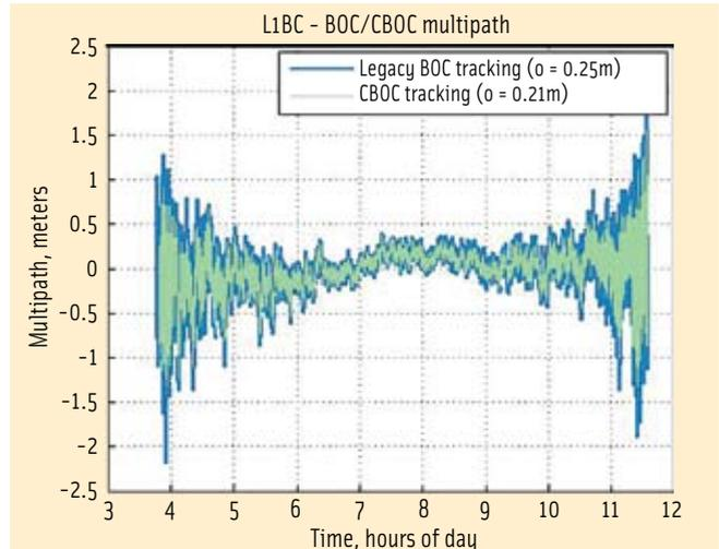
FIGURE 5 Simultaneous multipath time series of BOC(1,1) (blue) and CBOC (light green) obtained by the tracking of CBOC in two modes (comparison method [b]) for May 08 2008.
