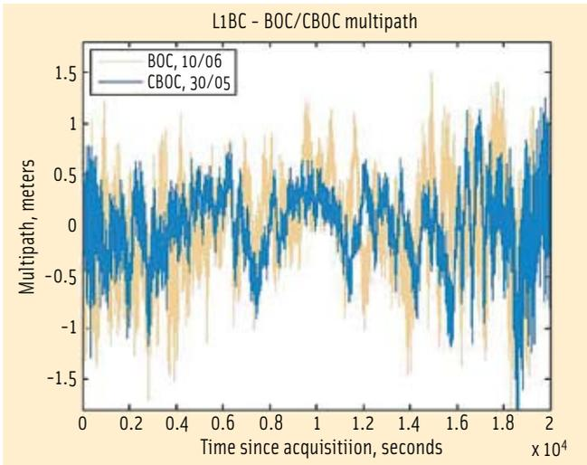
FIGURE 4 Multipath time series for L1BC for June 10, when BOC(1,1) was transmitted (results in light brown), are compared to May 30, when CBOC was transmitted (results in blue, comparison by method [a] described in article text).
