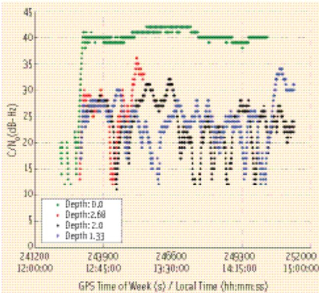
FIGURE 2 PRN 19  $C/N_0$  Measured in avalanche debris
