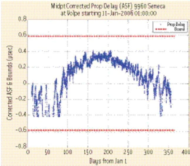
FIGURE 2 Propagation Delay and Bound at Volpe Center from Seneca, New York, transmitter (472 km)
