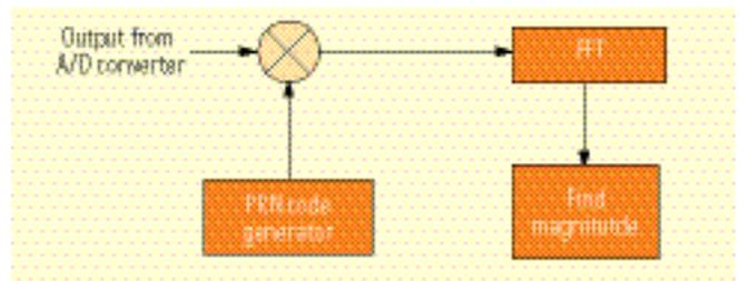
FIGURE 3 Parallel Frequency Search Receiver Architecture
