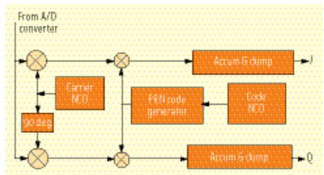
FIGURE 1 Serial-Search Receiver Architecture
