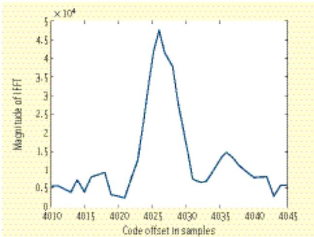
FIGURE 7 Detail of Correlation Peak Obtained using Parallel Processing
