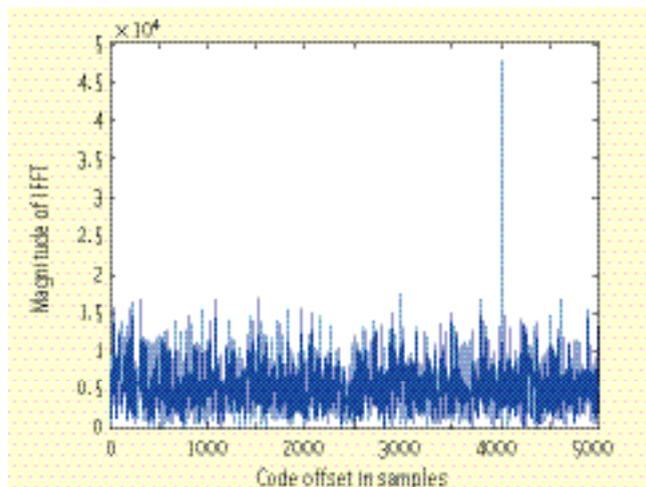
FIGURE 6 Code Offset Determination using Parallel Code Search Approach
