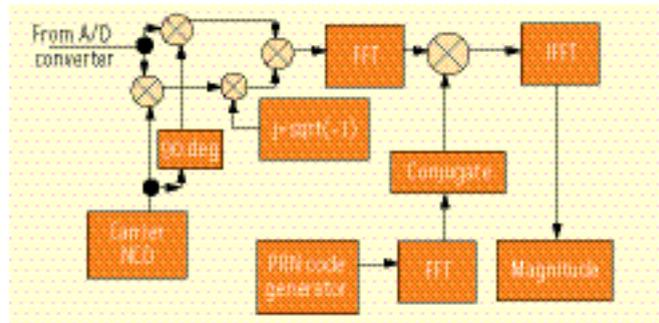
FIGURE 5 Parallel Code Search Receiver Architecture
