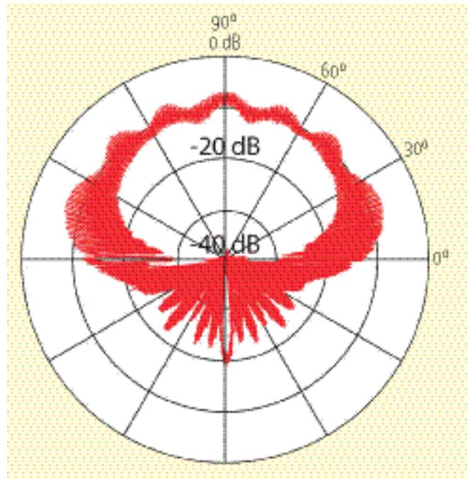
FIGURE 1 Patch Antenna Elevation Gain Pattern (-1 dBiC Peak)
